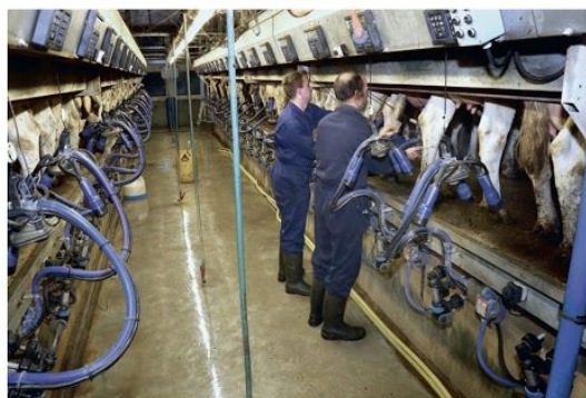
Evert always milks with help of a fellow worker. The cows are milked in a 2 x 20 side by side rapid exit parlor from DeLaval, with triangular fittings and head aeration from Milkrite.
